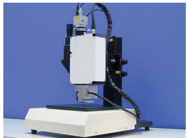
POST-H System : Controlling XY table by motorized stage
