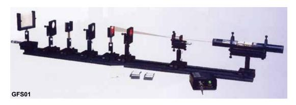
A tutorial system for Fourier Optics experiments, including Fresnel and Fraunhofer diffraction, spatial filtering, relay imaging, etc.
